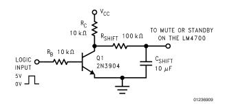
FIGURE 5. Level Shift Circuit
