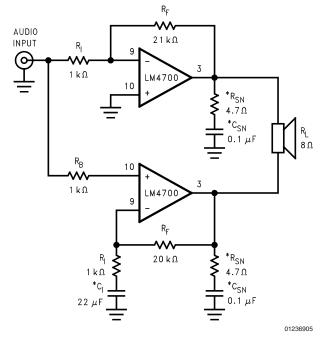
FIGURE 2. Bridged Amplifier Application Circuit
