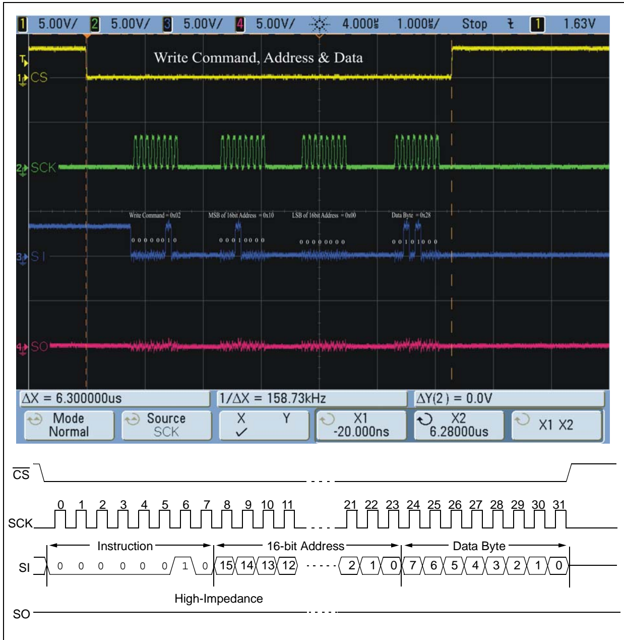
FIGURE 4: BYTE WRITE COMMAND, ADDRESS AND DATA
