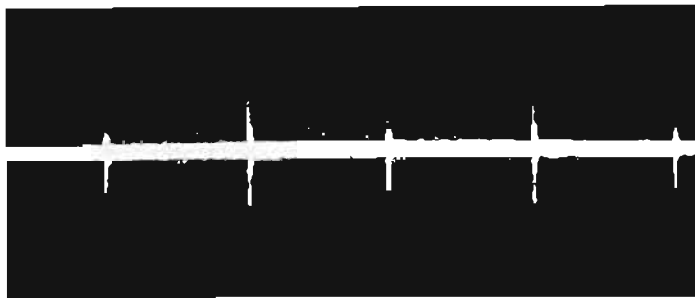
Figure 5. Reduced noise spikes in the circuit of Figure 4; vertical scale, 5 mV per division.
